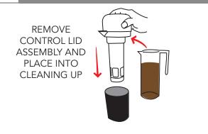
Place Control Lid Assembly(D) into the Cleaning Cup(H). For detailed cleaning instructions, refer to the 'Care and Cleaning' section on page 10.
