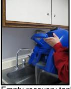
Empty recovery tank and solution tank.
