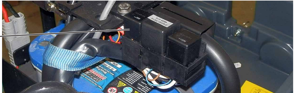
Brush motor relay (K1)
