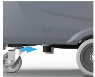
**11.** Daily: Empty the clean water tank using the solution tank drain knob under the machine.
