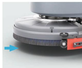
**3.** Place the brush or pad holder under the deck and lower the deck onto the brush or pad holder by pressing the pedal.
