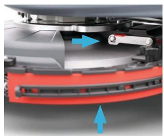
9. Lift the squeegee up by hand until it locks in up position and turn suction off for double scrubbing. To go back to working mode, use the red lever to release the squeegee and turn suction on again.
