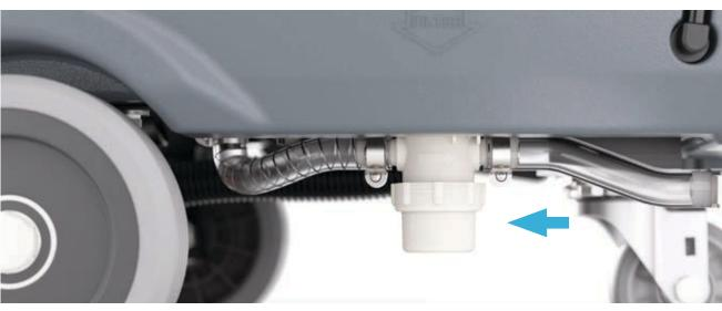
16. Weekly: Inspect the solution filter and clean if required.
