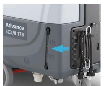
**6.** Check the solution level with the red ball on the left side of the machine.
