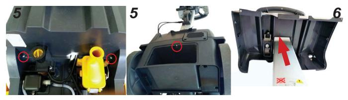
Take care when unplugging the fast-on connectors on the cables from the board; if overpulled, there is the risk of tearing off the fast-in connectors soldered to the board.
