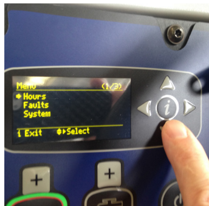
2. Press "I" scroll down to faults and press ">" button to view faults.
