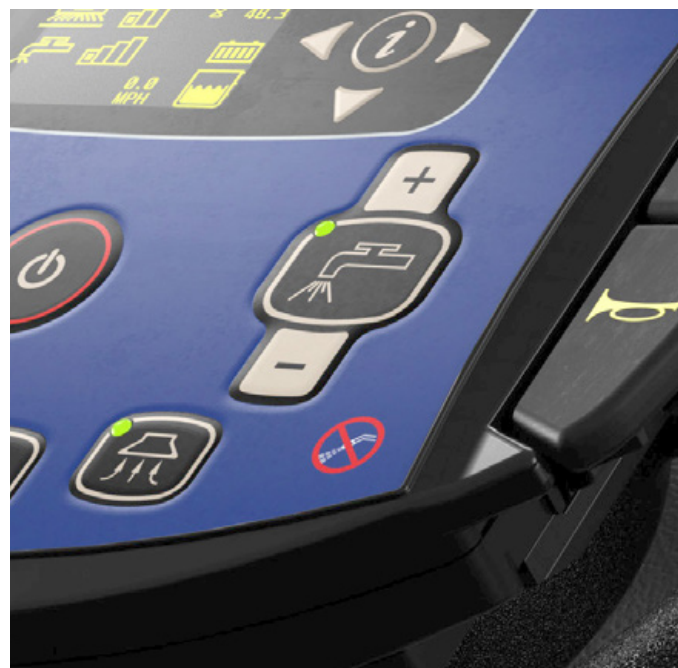
1. Verify that scrub parameters are correct for the required job. Increase pressure, solution and/or detergent concentration as needed.
