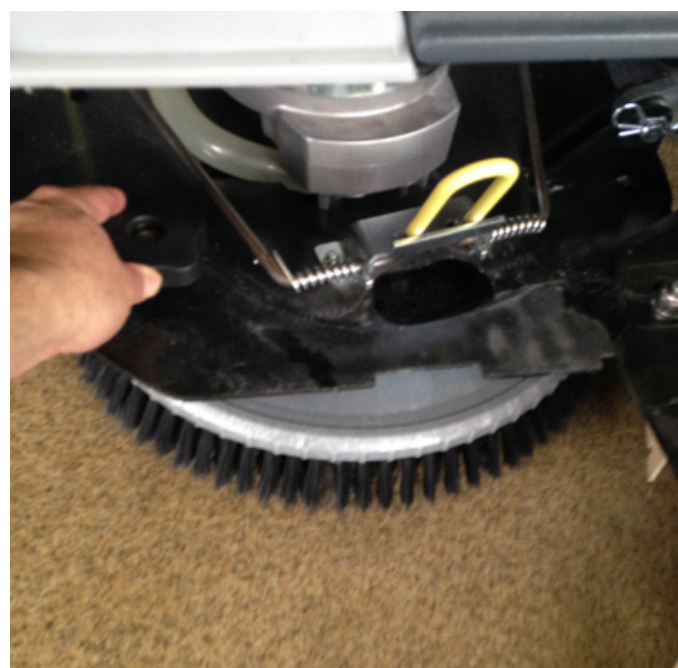
1. Remove side skirt assembly and verify brush installation and condition.
