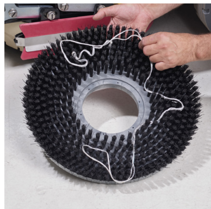
3. Turn brushes counter clockwise and check if there are external materials avoiding brush rotating.
