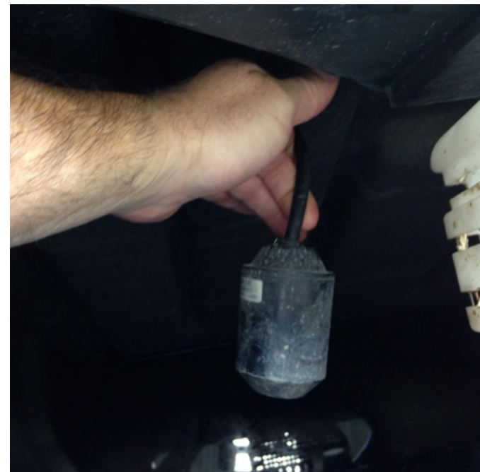
2. Inspect recovery tank float switch operation.
