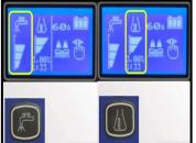
Adjust water flow (as needed). EcoFlex Chemical Settings for dilution ratio (must have yellow super-user key).
