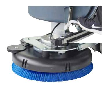
6. Place the appropriate brush or the padholder under the deck. Lower the deck by pressing the pedal.
