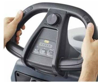
10. Begin scrubbing by placing hands on the touch sensors on the handlebar.
