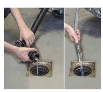
14. Empty the recovery tank with the flex hose. Then empty the solution tank using the transparent hose.
