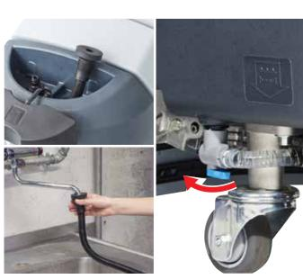
2. Fill solution tank with clean water (do not exceed 40 °C / 104°F). Ensure the solution valve under the machine is in the open position.
