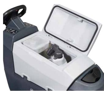
20. Park the machine with the recovery tank cover in the open position for ventilation.
