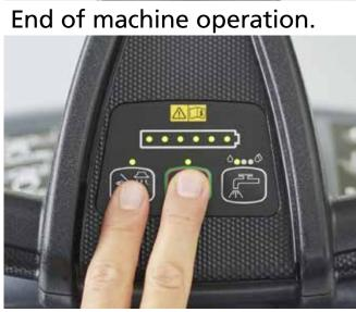
13. Lift the squeegee and press the main button to turn machine off. Lift the brush deck by pressing the pedal. To disengage the brush, press the vacuum button and the main button simultaneously for 1 second.
