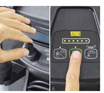
7. If machine has a ignition key first set it to"I", press the main button once to activate the machine. Battery indicator will turn on.
