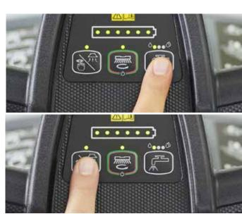
12. Press the solution button to adjust the solution flow to the cleaning needs. When the LEDs are off, the solution flow is off. If necessary press the Quiet mode button for extra low sound level (LED will flash).
