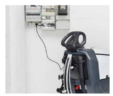
1. Disconnect the on board battery charger cable from the electrical outlet.
