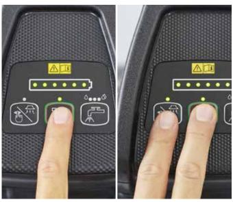
8. Press the main button again (with LED on) to start the machine, press the vacuum button and the main button simultaneously for 1 second to engage the brush "click on" to the deck.
