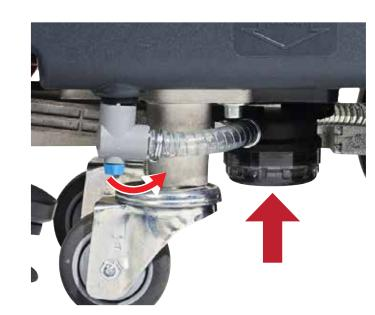
16. Clean the filter: A) Close the solution valve under the machine. B) Remove the transparent cover and the gasket, then remove and clean the filter inside. C) Reassemble the filter.
