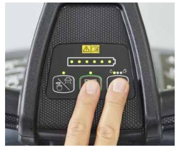
9. For sensitive floors the brush/pad can be made "pre-wet" with solution before starting to avoid marks. Press the main button and the solution button simultaneously for 10 to 20 seconds before starting to scrub.
