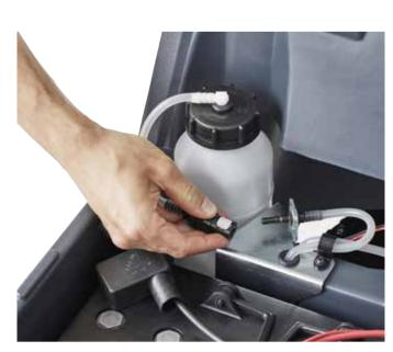
3. For machines equipped with the detergent mixing system, fill the bottle with a suitable detergent and attach the hose. For machines without this option, add the manufactures recommend dosage to the solution tank.
