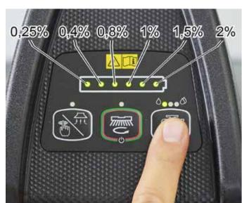
4. For detergent system option, select the percentage of detergent by pressing and holding the solution button for 2 seconds, than toggle to the desired setting by pushing the solution button.
