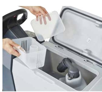
15. Empty the debris catch cage and wash the recovery tank with clean water.
