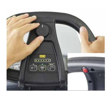
11. For drive models, adjust the maximum speed with the speed adjustment dial. To reverse, press the red button on the handle together with one hand on any of the touch sensors.
