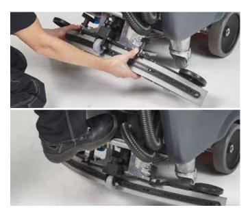
5. Install the squeegee and fasten it with the fly wheel. Lower the squeegee by pressing the pedal.
