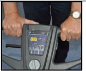
Enable push-button and lever to engage brush/pad holder then release.
