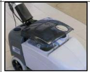
Lift recover tank lid to allow inside of the tank to dry.
