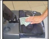
Wipe exterior of machine with a damp cloth.
