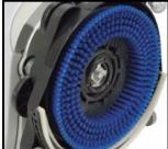
Remove, clean and inspect brush or pad. Rinse with warm water. Hang to dry. Replace if needed.
