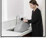
Fill machine with appropriate solution (temperature should not exceed 130 °F).
