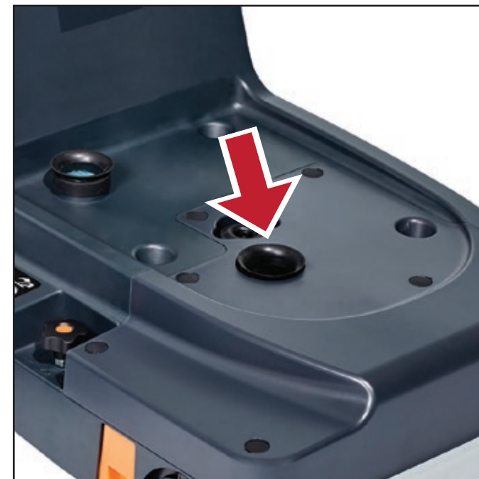
3. Rinse the inside of the duct recovery hose with water.
