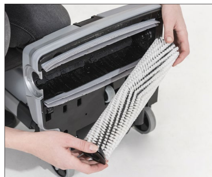
18. Remove the cylindrical brush by turning the side knob clockwise.
