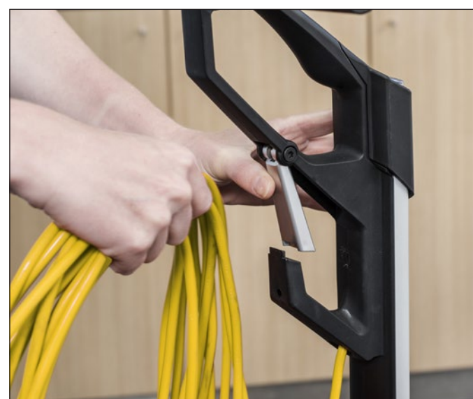
14. Disconnect the power plug from the electrical socket and rewind the cord starting at the machine and place it in the cord holder.
