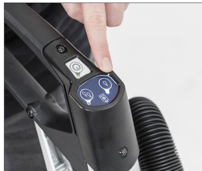
8. Press one of the solution buttons, according to the type of cleaning to be performed: 1 drop - normal cleaning 2 drop - heavy duty cleaning
