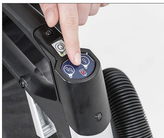
11. The red LED blinks when the machine is getting low on solution and has a fixed light when empty. Empty the recovery tank and refill the solution tank to continue working.
