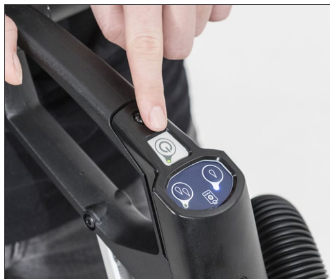
7. Press the start/stop button to start the machine.
