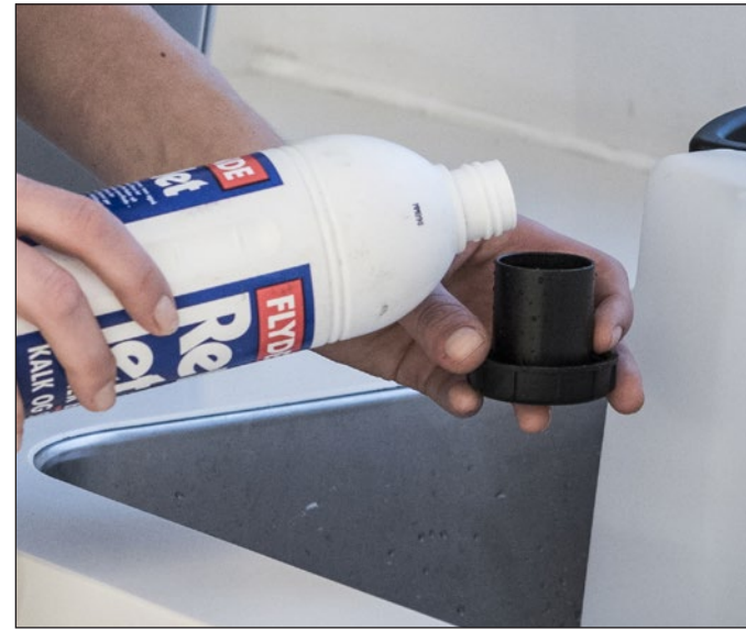
3. The tank cap can be used for dosing the detergent. One full cap is 30 ml giving 1% detergent of the 0.8 gal (3 L) tank capacity. (*)
