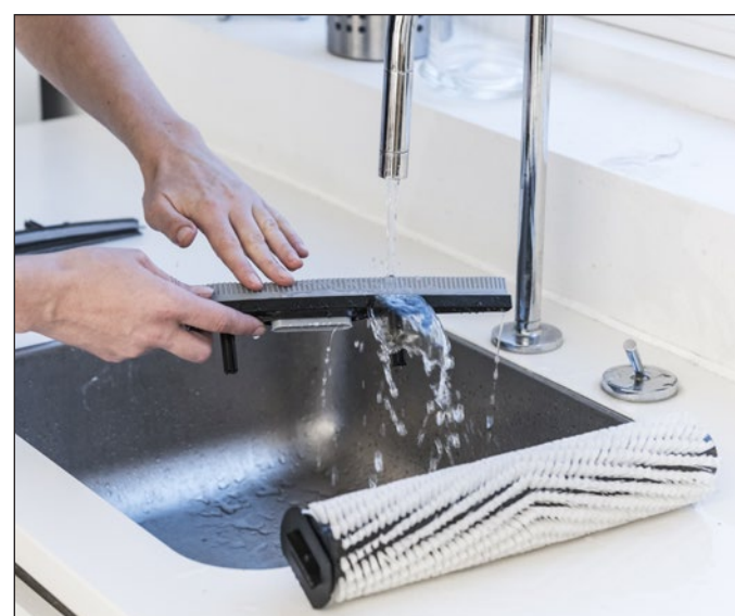
19. Clean the squeegee bars and the cylindrical brush with water. Check for wear and replace when necessary.
