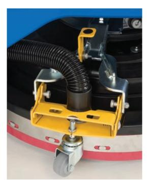
1 Check to make sure the vacuum hose is connected to the squeegee.
