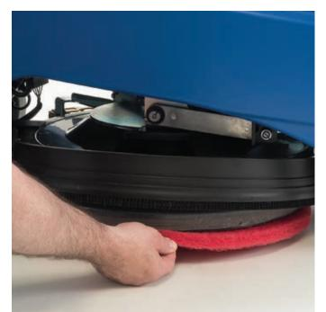
1 Check to see if the pad is correctly installed and not worn out.
