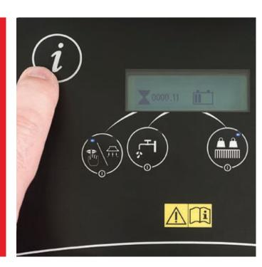
**1** Check the battery charge gauge (and if necessary re-charge).
