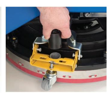
3. Check to make sure the vacuum hose is connected to the squeegee.
