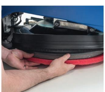
5. Install the pad on the deck.
