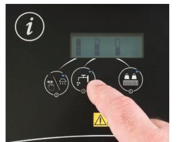
9. Adjust the desired water flow.
