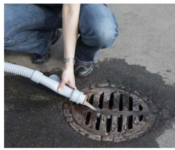
13. Empty the recovery tank with the squeezable hose.
