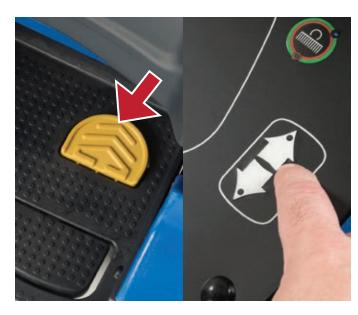
12. Press the forward foot pedal, then select the direction and start operating the machine.
