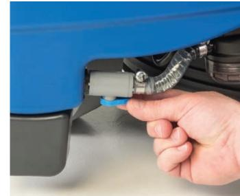
14. If necessary, empty the solution tank through the solution valve and clean the filter net.
