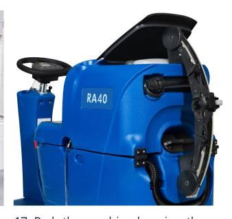
17. Park the machine keeping the recovery tank cover open and hang the squeegee.
