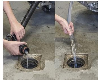
11. Empty the recovery tank with the hose. Then empty the solution tank with the transparent hose.
