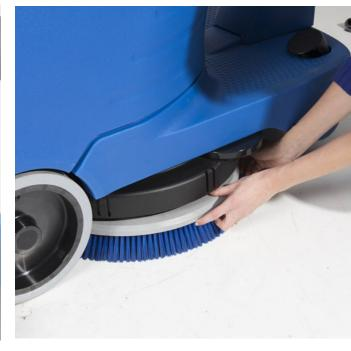
2. Check if the brush is correctly installed and not worn out or if there are external materials preventing brush rotation.
