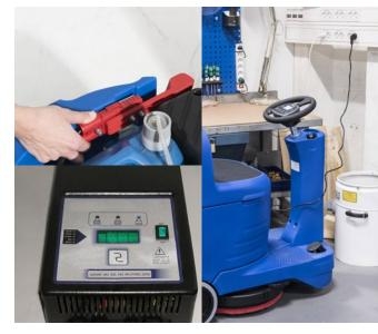
16. Charge the batteries: Connect the battery charger cord to the electrical outlet.
