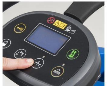
9. If necessary press the vacuum button for stop/start vacuuming.
