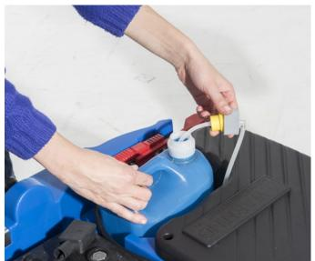
3. For machine equipped with Chemical 4. Install the squeegee and fasten it Mixing system: Mount the tank with a detergent suitable for cleaning machines (highly concentrated and low foaming detergent)
