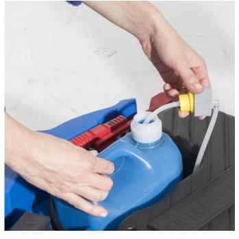
Check to make sure the Chemical Mixing System is clean. Eventually purge the system.
