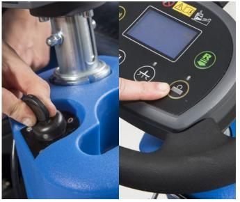
6. Insert and rotate the operator key, then start the machine by pressing the One-Touch button. To engage the brush, slightly press the pedal speed and then release it.
