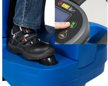
7. Push the drive pedal to start cleaning. Adjust the speed by applying pressure to the drive pedal. For the reverse mode press the green button.
