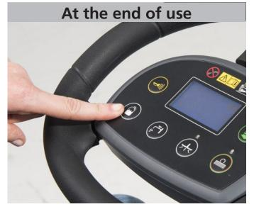
10. Machines with Chemical Mixing System: Always turn off the detergent 2 minutes before finishing by pressing the detergent button to rinse out detergent from the system and brush before handling and cleaning.
