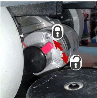
4. Check if the electromagnetic brake is locking.
