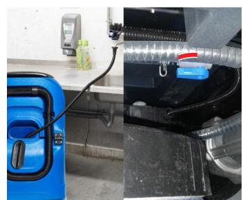
2. Fill the tank with clean water. The water temperature must not exceed 40° C.
