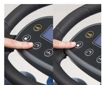
8. To change the solution flow level push the solution button and change the flow level according to desired cleaning performance and application.
