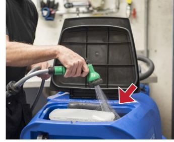
12. Empty the debris tray and clean/ wash the recovery tank inside.
