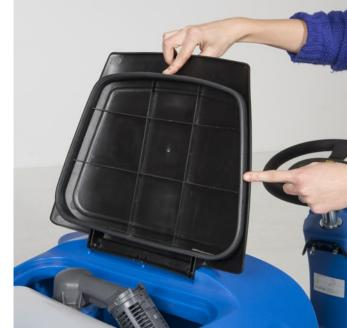
4. Check to see if the lid gasket is in good and working condition and sealing when the lid is closed.
