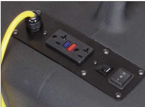
2 position switch and daisy-chained outlets
