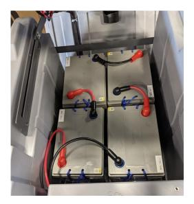
**Hint:** Paint a thin layer of metal-free lubricating oil or protective spray on the connected wiring to avoid battery corrosion.
