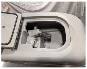
• Check the abrasion conditions of the skirt section of the brush head
