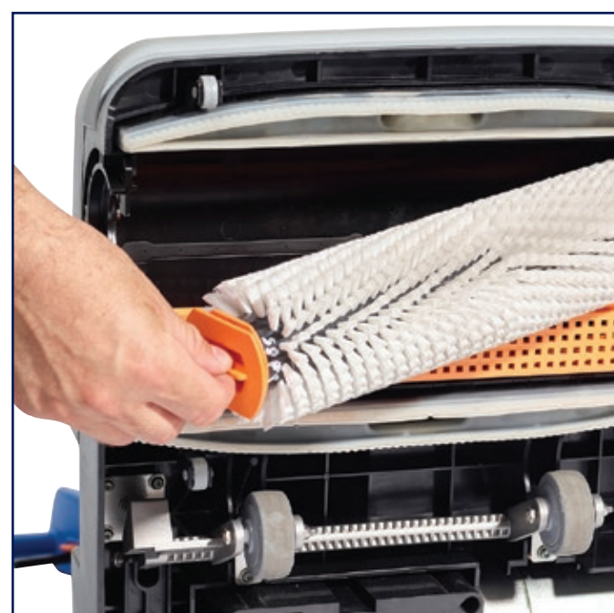
2. Check for brush wear, and make sure that it is installed correctly.
