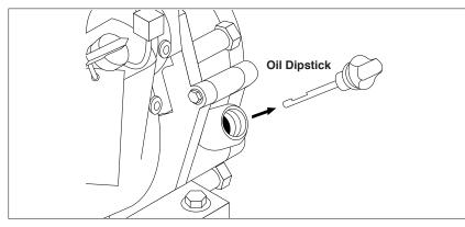
**STEP 1:** Check engine oil level. Oil level should be level with the bottom of the oil filler neck. Be sure the machine is level when checking the oil level. (Refer to the engine's operating manual included with machine.) We recommend that the oil be changed after the first 5 hours of use, then once every 50 hours. **Note:** Improper oil levels will cause low oil sensor to shut off engine. **IMPORTANT! Do not run engine with high or low oil levels as this will cause engine damage.**
