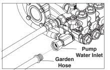
**STEP 7:** Check inlets filters, remove debris, then connect the garden hose to pump water inlet. *CAUTION: Do not run the pump without water or pump damage will result.*
