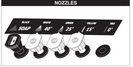
The four color-coded quick connect nozzles provide a wide array of spray widths from  $15^{\circ}$  to  $40^{\circ}$  and are easily accessible when placed in the convenient rubber nozzle holder, which is provided on the front of the machine.
