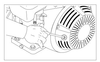
**STEP 9:** Pull the starter grip. If the engine fails to start after 2 pulls, squeeze the trigger gun to release pressure and repeat step. Return starter gently. After the engine warms up enough to run smoothly, move choke to run position and throttle to fast position.
