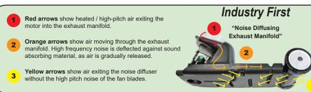
Mosquito's exclusive "Noise Diffusing Exhaust Manifold" suppresses high-frequency sound with its noise-canceling technology. Motor exhaust is directed through exhaust grates which redirects sound waves while gradually releasing exhaust. No back pressure is generated from this device as it scrubs 8dB and 11dB sones from the final exhaust. This is an industry first and the beginning of a new generation of extractors fromMosquito.
