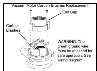
If armature commutator is grooved, extremely pitted or not concentric, the motor will need to be replaced or sent to a qualified service center.
