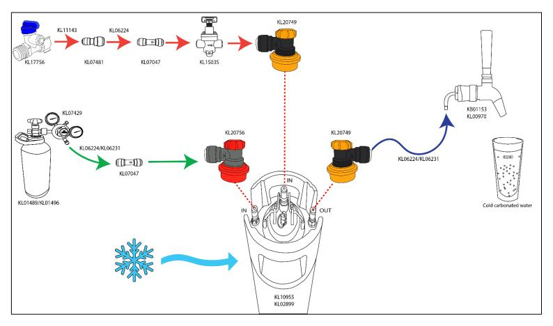
There are a number of different ways that you could setup the soda carbonator differently to how it is described above. Pre-chilling the water prior to it entering the carbonator keg will allow for a greater throughput of carbonated water. If you are going to be consuming more than 10 Litres per day it is suggested that you pre-chill the water.
