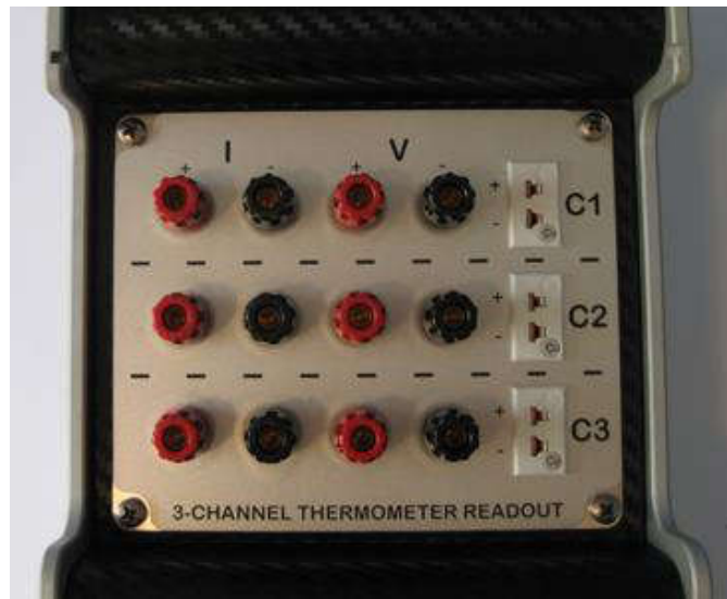
Figure 2: Connectors for the connection of thermometer probes on main channels
