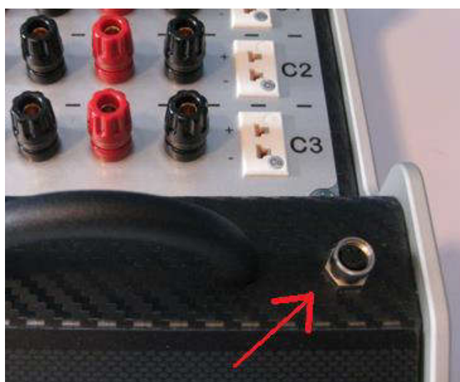
Figure 8: Ambient probe connector with plastic protective plug removed
