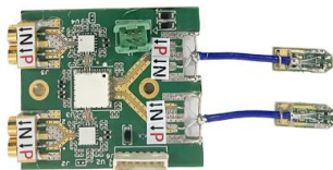
P4012-CTLE (UFS4.0 Compatible Solder Probe tips with CTLE with sense resistor connected.)
