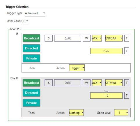
PGY-RFFE-EX-PD supports auto, simple, and advanced trigger capabilities. The analyzer can trigger on any of the Protocol packets such as Ext. Reg. Write, Ext. Reg, read and so forth message. Advanced Trigger provides the flexibility to monitor multiple trigger conditions and can set multiple state trigger machines.
