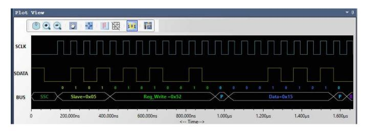
The timing view provides the plot of SCLK and SDATA signals with a bus diagram. Overlaying of Protocol bits on the digital timing waveform will help easy debugging of Protocol decoded data. Cursor and Zoom features will make it convenient to analyze Protocol in the timing diagram for any timing errors.
