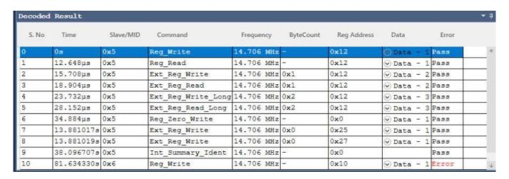
The protocol window provides the decoded packet information in each state and all packet details. The selected frame in the Protocol listing window will be auto-correlated in the timing view to view the timing information of the packet.
