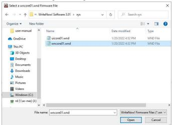
For WriteNow! programmer the firmware filename is wncore01.wnd
