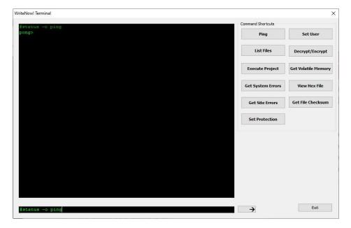
Commands can be sent (and answers received) using any terminal application. For your convenience, the Project Generator application includes a Terminal window that will simplify the communication with the instrument. Just select **Tools > WriteNow! Terminal** to open the Terminal window.
