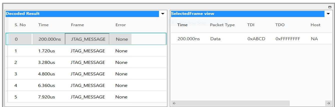
Protocol window provides the decoded packet information in each state and all packet details with error info in packet. Selected frame in Protocol listing window will be auto correlated in timing view to view the timing information of the packet.
