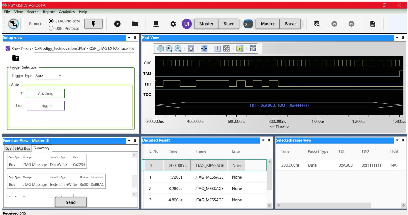
Multidomain View provides the complete view of JTAG Protocol activity in single GUI. User can easily setup the analyzer to generate JTAG traffic using a GUI or script. User can capture JTAG Protocol activity at specific event and decode the transition on JTAG bus. The decoded results can be viewed in timing diagram and Protocol listing window with autocorrelation. This comprehensive view of information makes it industry best, offering an easy to use solution to debug the JTAG protocol activity.
