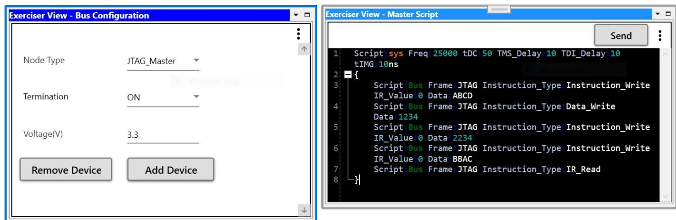
PGY-JTAG-EX-PD supports JTAG traffic generation using GUI and Script. User can generate simple traffic generation using the GUI to test the DUT. Script based GUI provides flexibility to emulate the complete expected traffic in real world including error injections. In this sample script user can generate JTAG traffic as below:
