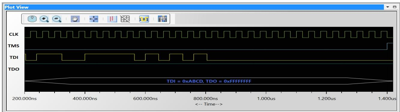
Timing view provides the plot of CLK, TMS, TDI and TDO signals with bus diagram. Overlaying of Protocol bits on the digital timing waveform will help easy debugging of Protocol decoded data. Cursor and Zoom features will make it convenient to analyze Protocol in timing diagram for any timing errors.
