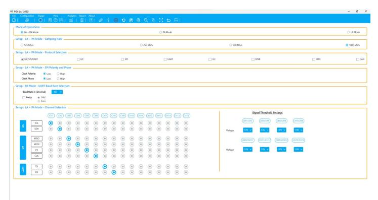
Users can easily configure the Logic Analyzer for embedded interfaces by either selecting Logic Analysis (LA) mode or Protocol Analysis (PA) mode or a combined (LA+PA) mode. This ensures a quick and easy way to configure the product and look at complex problems at system level either in Logic Analysis (State Analysis, Timing Analysis) or Protocol decoding or both. Save and Recall capability ensures designers can recall their custom setup details.
