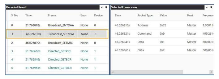
The protocol window provides the decoded packet information in each state and all packet details with error info in the packet. The selected frame in the protocol listing window will be auto-correlated in the timing view to view the timing information of the packet.
