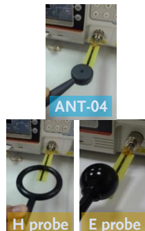
ANT-04: higher sensitivity than H probe and E probe
