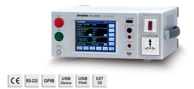
The GLC-9000, leakage current tester, is used to perform leakage current (or called touch current) tests on general purpose electric (IEC 60990) equipment. This tester engages with nine measurement networks (or called Measuring Device) to provide the simulation of human body whilst the EUT (equipment under test) is taking a leakage current testing , in compliance with the specific standards or regulations such as IEC, UL, JIS...etc..
