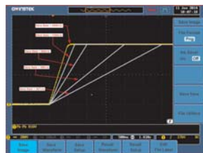
The Adjustable Rise Time of the PSW 800V Module
