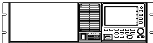
GRA-439-E Rack Mount Diagram (ASR-2000R)
