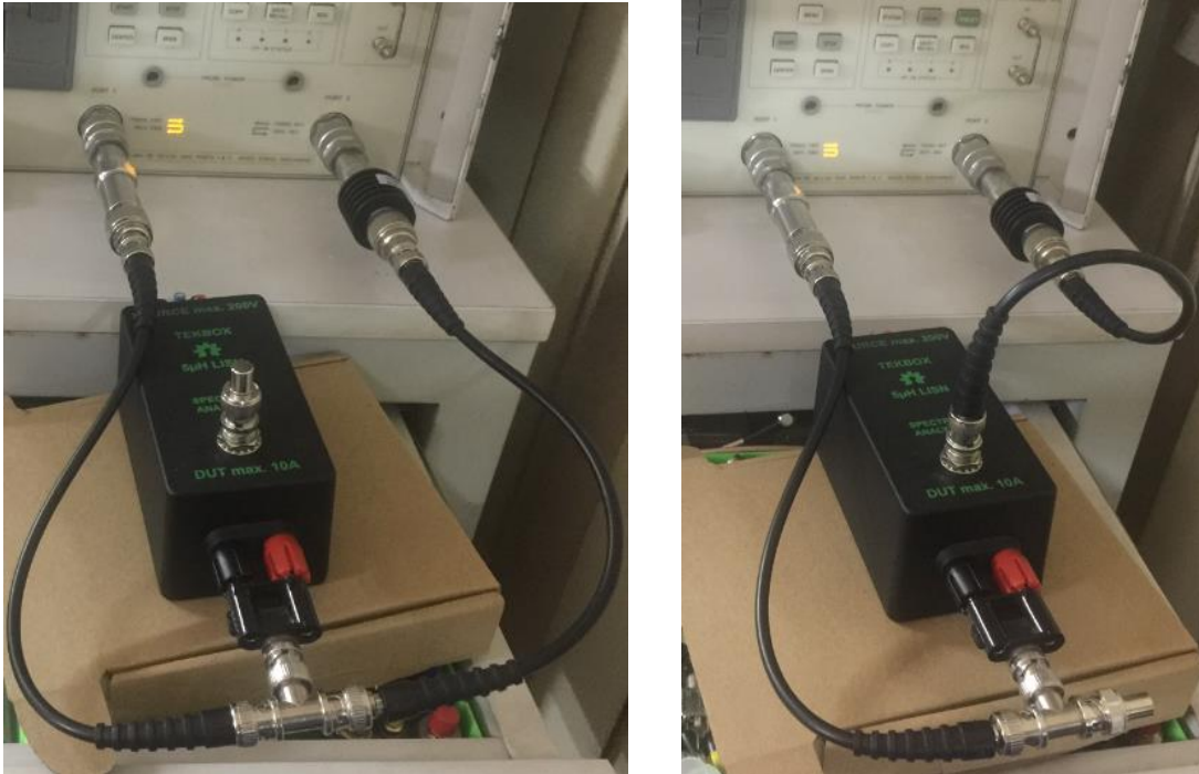
Picture 3: LISN insertion loss, left – calibration set up, right – measurement set up
