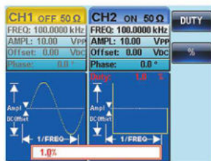
1% Duty Cycle of Square Wave
