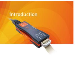
JTAG Live® is the breakthrough product for design and test engineers to debug boards too crowded for traditional probing. JTAG Live enables you to sense signal levels on prototype PCBs, verify proper continuity between pins or groups of pins, and check basic operation.
