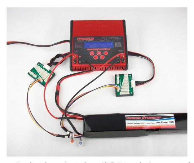
Now you will need to configure each port to charge a 5S LiPo battery at the charge current rate of your preference. We suggest configuring one of the ports correctly, then moving to the second port to configure it correctly. Then start the charging process on the last port you configured then switch to the other port and start the charge process accordingly.
