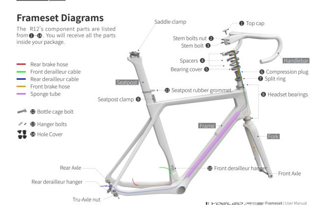
**Brake & Gear Housing Routing - Mechanical** Route the housing into the down tube of the frame from the hole where each house comes out Please measure the correct length of the brake and shifter housing before cutting. Rear brake hose Front derailleur cable Rear derailleur cable Front brake hose Sponge tube Rear derailleur hanger Hanger bolts 3Nm Cable grommet **4** Tru-Axle Nut
