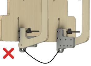
NOTE: The bracket "assistance rings" are only to be loaded VERTICALLY, with a capacity of 50 lbs. Never load them horizontally or connect the two rings.
