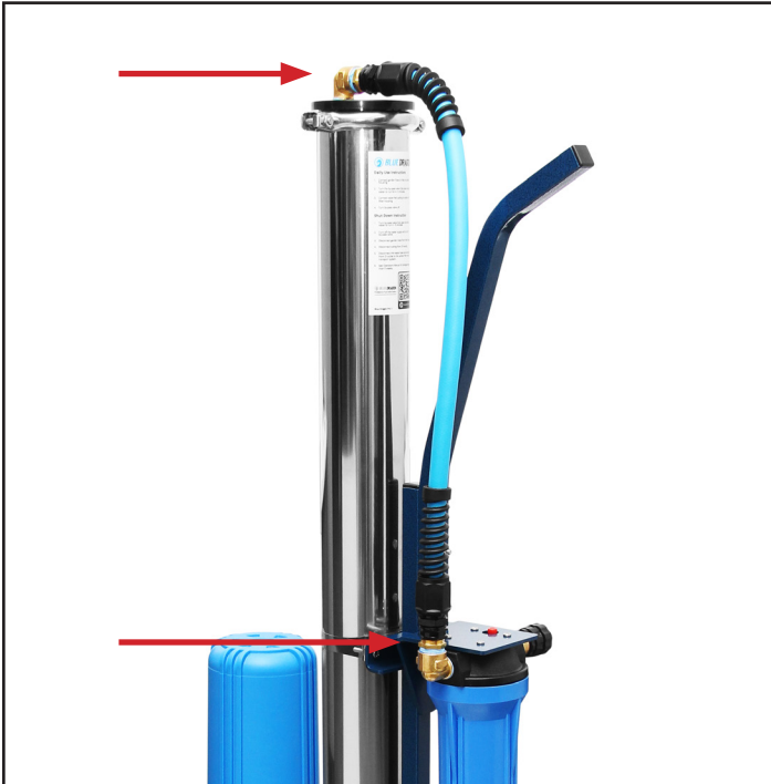
5. Mount the 5/8 light blue hose from the cap to the carbon filter housing outlet.
