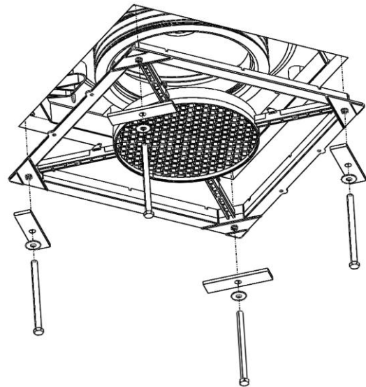
Figure 9- Assemble Bolt, washer & bar into duct & brace
