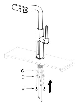
Install the mounting hardwares (C-E) in sequence according to the figure below, and fix the faucet on the countertop.
