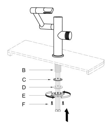
Install the mounting hardwares in sequence.
