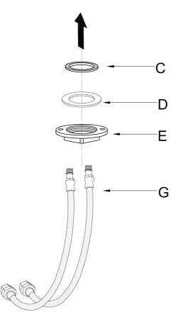
Install the hot and cold water pipes (G) through the mounting hardwares and screw in tightly.
