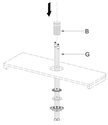
Swivel the hot and cold water pipes (G) through threaded metal pipe (B) into the faucet body.
