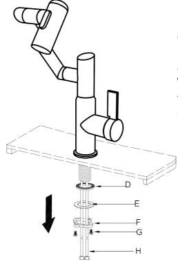
Pass the rubber gasket (D), metal gasket (E) and mounting hardware (F & G) through the metal pipe in turn and tighten them.
