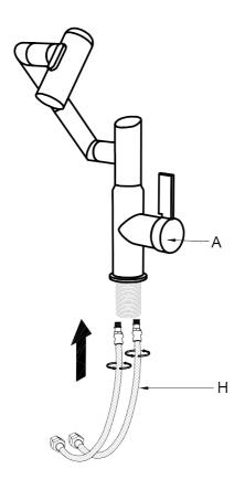
Swivel the hot and cold water pipes (H) into the faucet body (A).
