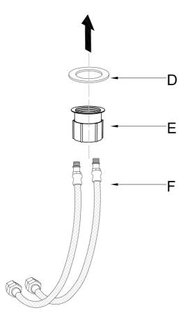
Install the hot and cold water pipes (F) through the mounting hardwares (E&D) and screw in tightly.
