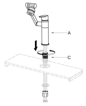
Pass the rubber gasket, metal gasket and mounting hardware through the metal pipe in turn and tighten them.
