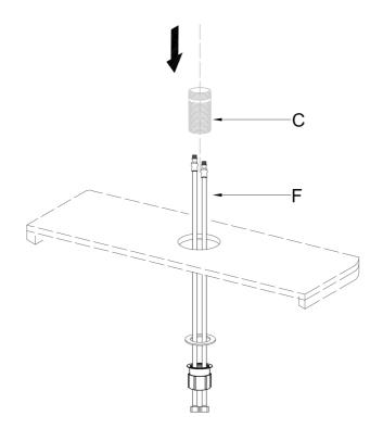
Swivel the hot and cold water pipes (F) through threaded metal pipe (C) into the faucet body.
