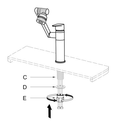
Install the mounting hardwares in sequence.
