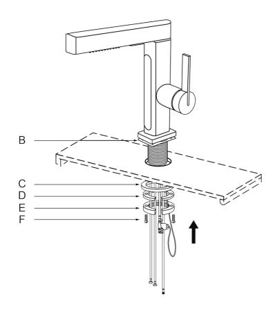
Install the mounting hardwares (B-F) in sequence according to the figure below, and fix the faucet on the countertop.
