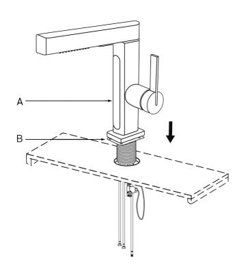
Shut off the water supply. Remove the old faucet. Clean the mounting surface. Thread the faucet through the hole and install it on the countertop.
