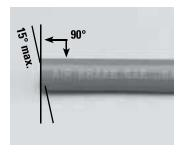
Using a tube cutter, make a square cut edge (maximum 15° cutting angle allowed).
