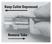
2. Depress collet head using fingers or tube-release tool to release grip on tubing.
