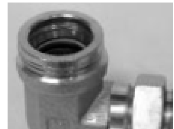
Figure 5 – Properly Assembled O-ring & Back-up ring
