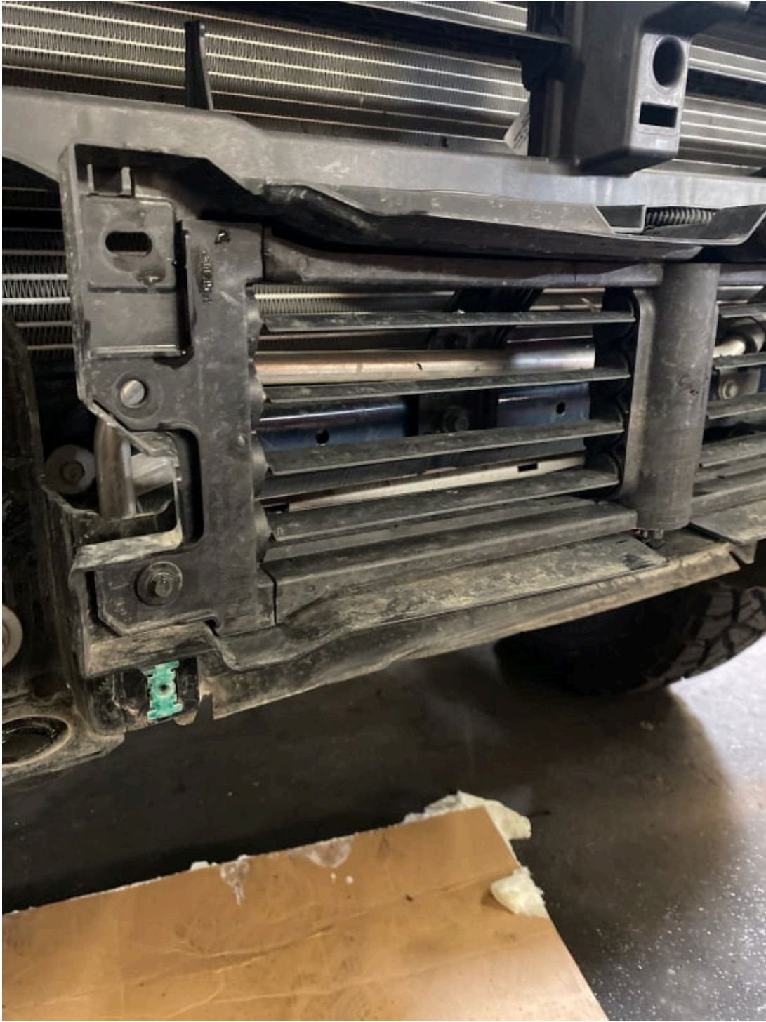
SHUTTER RELOCATION IMAGE- SHUTTER SYSTEM GETS RELOCATED UP, USING THE EXISTING MOUNTS
