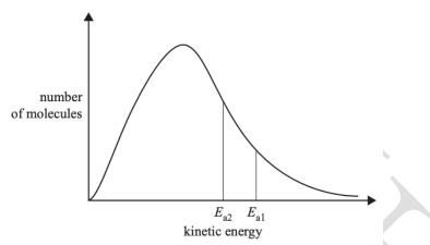
The diagram above represents the distribution of kinetic energy in a sample of gaseous reactant molecules. Activation energy  $E_{a1}$  can be changed to activation energy  $E_{a2}$ . This change increases the reaction rate.
