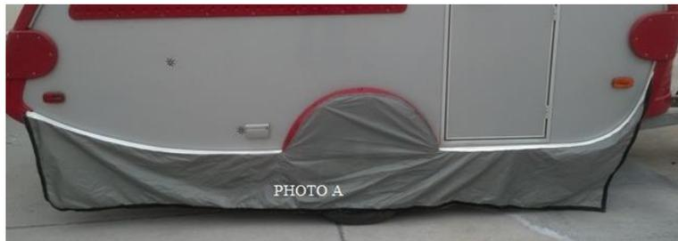
4. **Starting** at the rear of the trailer, slide the keder cord into the keder rail on the passenger side of your trailer. Make sure that the keder cord is able to feed freely into the rail as you pull the Tent towards the front of the trailer. The keder cord should fit completely into the rail, with little or no excess hanging out on either end.
