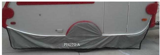
4. **Starting** at the rear of the trailer, slide the Tent keder cord into the keder rail on the passenger side of your trailer. Make sure that the keder cord is able to feed freely into the rail as you pull the Tent towards the front of the trailer. The keder cord should fit completely into the rail, with little or no excess hanging out on either end.
